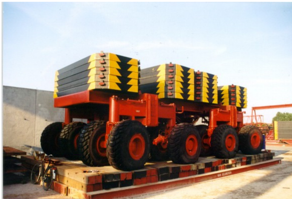
480t ballast on wheeled carrier (1.000t on ring)
